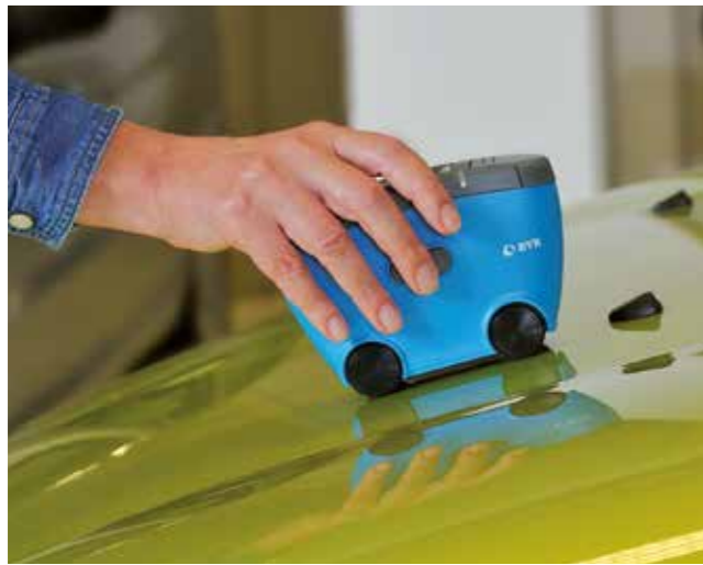
Measuring surface quality (Wave Scan Dual)
