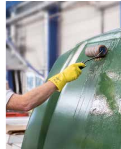
Pre-application of the 1. Layer resin
