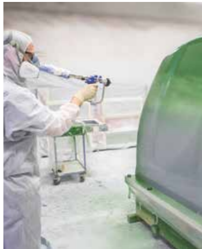
Applying gelcoat by spraying
