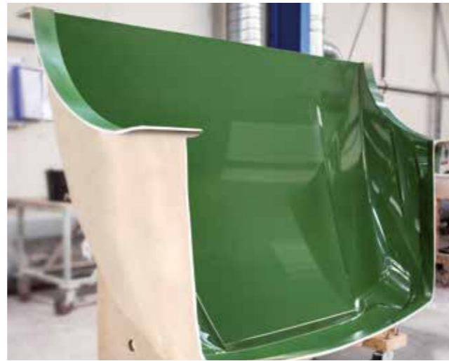
Mould for the alcove of a camper
